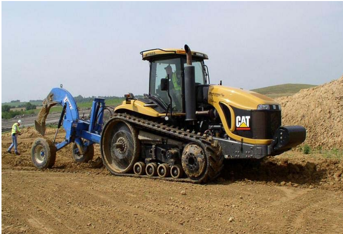
Caterpillar track type tractor prepares for ripping demonstration.
